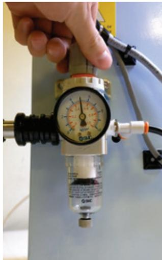
Lift the knob to unlock the regulator.
