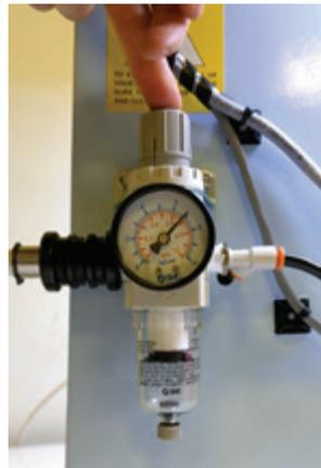
Once getting to 7 kg correctly, press the knob to lock the regulator.
