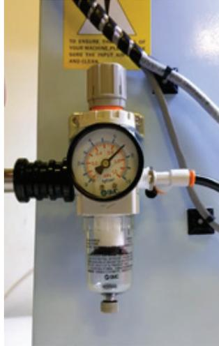
The pressure regulator must always be at 7 kg.
